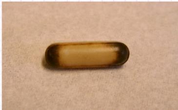
Magnetic stir bars are highly chemically inert, small magnetic bars. Most heaters have a built-in magnet which can rotate. Through this rotation the magnetic stir bars are spun and the solution the magnetic stir bar is in is homogenized.
